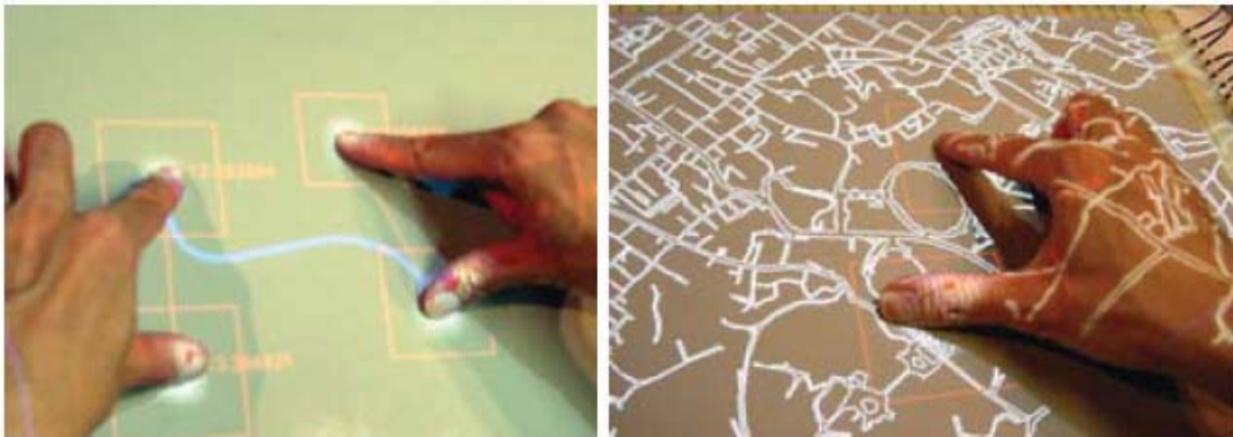
Figure 12: Examples of uses of multiple-finger interfaces: left: curve editing. right: a map browsing system. The user can use one finger for panning, or two or more fingers for simultaneous panning and scaling.
